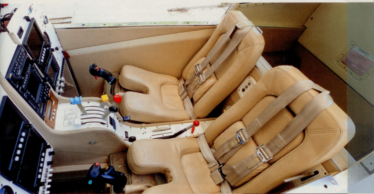
Two of the three screens for the Grand Rapids Technologies Horizon 1 display are in front of the pilot (top left); the control stick has buttons to transmit, disconnect the autopilot, record and display incoming radio transmissions, flip radio frequencies, select the radio transmitter, and squawk ident; the uncluttered panel with a three-screen Horizon 1 EFIS display (below left); the 41-inch-wide cabin is luxurious (above).
